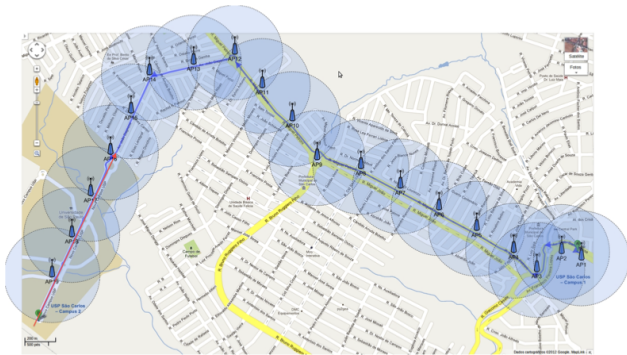
Figure 20: A map with the estimated provision of routers (named AP1 to AP19) along the path.
