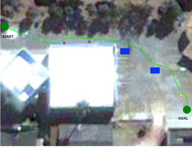
Figure 12: Vehicle’s path (green segment) provided by the MTi-G sensor. Red cylinders are the traffic cones, blue rectangles the cars and yellow circle a person.
