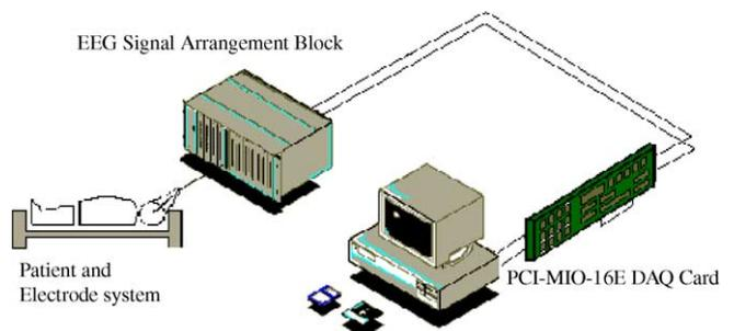
Fig. 1. Scheme of the EEG data acquisition system.
