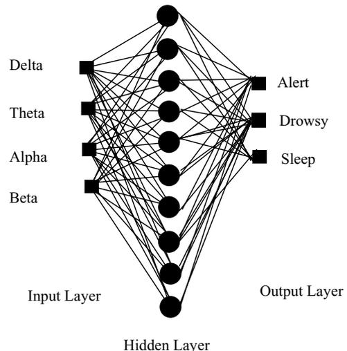
Fig. 4. Multi-layered neural network model.
