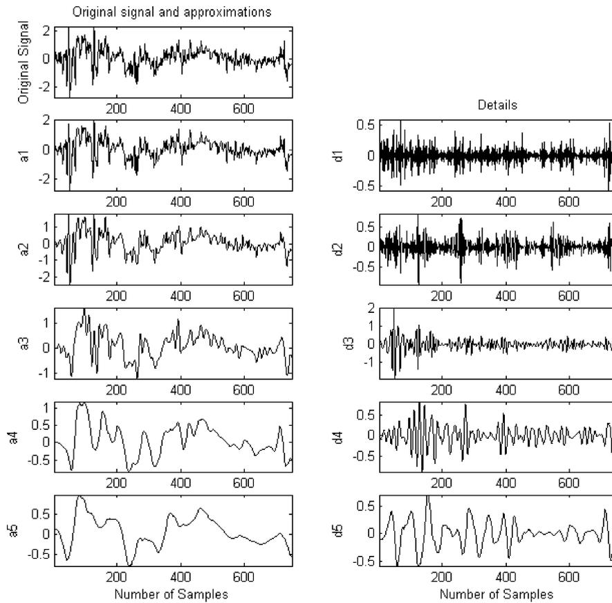
Fig. 3. Daubechies order 2 wavelet transform of an EEG signal.
