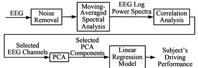
Fig 2: Analysis flowchart of the EEG signals.
