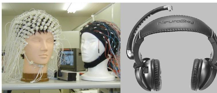
**Figure 2.2:** Traditional cap with a grid of electrodes vs. new type, single electrode headset (NeuroSky).
