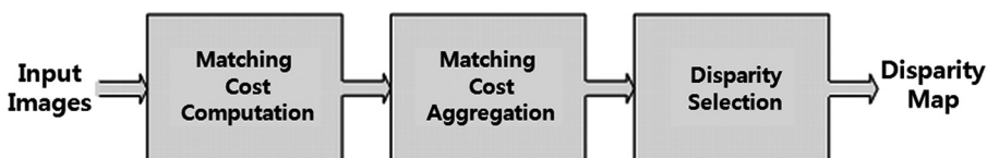
Figure 8. Generalized block diagram of a hardware implementable stereo correspondence algorithm.
