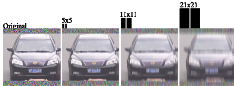
Figure 2. The original vehicle image and motion blurred images convolved with kernels of different size.
