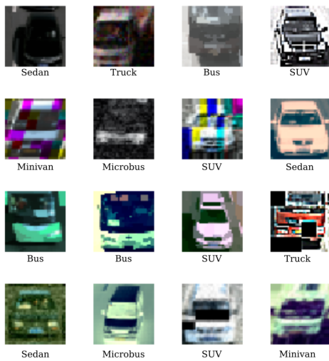
Fig. 3. Some resized samples of the augmented BIT-Vehicle dataset. There are a random number of variations in each image such as translation, rotation, blur, sharpening, brightness, and saturation.
