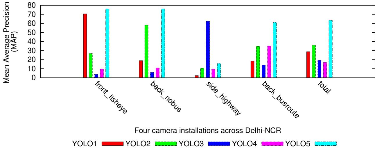
Figure 3: Mean Average Precision (MAP) of the five object detection models on the five test sets (one from each of the four camera installations and a fifth combined test set)
