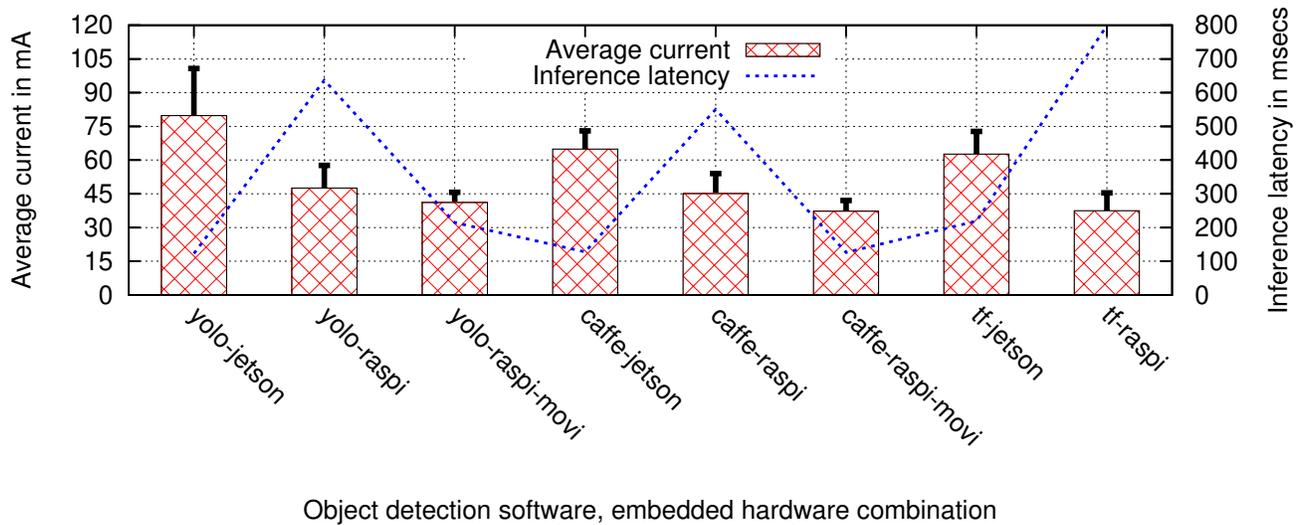
Figure 5: Inference latency and energy of object detection DNN software on embedded hardware platforms
