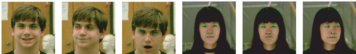
Figure 8: User-independent facial tracking: the red arrow denotes the position and orientation of the head and the green dots show the positions of the tracked points.
