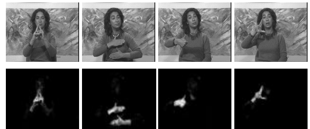
Figure 4. Result of combining color and motion into one probability map. Intensity corresponds to probability.
